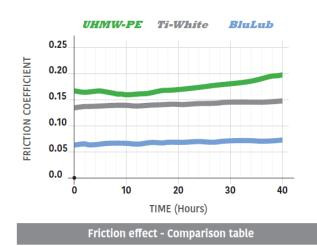
BluLub is a super-performance compounded UHMW-PE material with the latest generation of solid lubricants, contributes to improve PV-properties, especially in applications with limited lubrication, higher speeds and/or higher loads.
