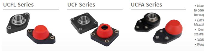
Housing in reinforced polyamide, with higher load capacity and good resistance to corrosive chemicals such as water, oils, petrol and alcoholic beverages. All our bearings can be used at temperatures between 0°C and +80°C.
