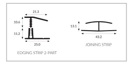
Ceiling profiles are used to create a strong, watertight seal for the ceiling planks to connect into.
