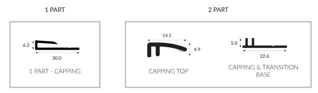
Capping profiles are used to create a watertight seal between the sheet and the ceiling/flooring.
