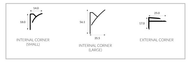
Corner profiles are used to create a watertight seal between two corner sheets.
