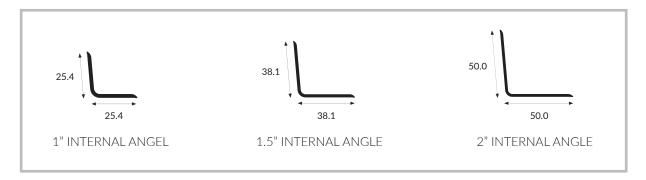
Internal angle profiles are used embedded corners to create a watertight corner seal.
