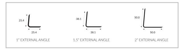
External angle profiles are used on extruded corners to create a watertight corner seal.
