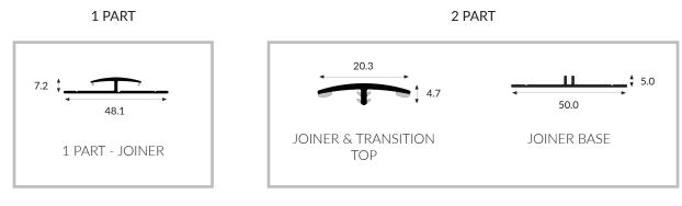
Joiner profiles are used to create a watertight seal between the sheet and the ceiling/flooring.
